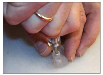
**13.** Rest the mould on a piece of wood or some other material when making the last part of the sound canal.
