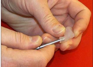
**12.** Force the tip of the earmould into a straight angel and drill the sound canal, using the special drill.
