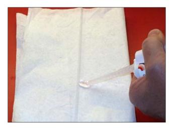
5. When using a new cartridge, always dispose of the first two cm of the material on a piece of paper/Kleenex.
